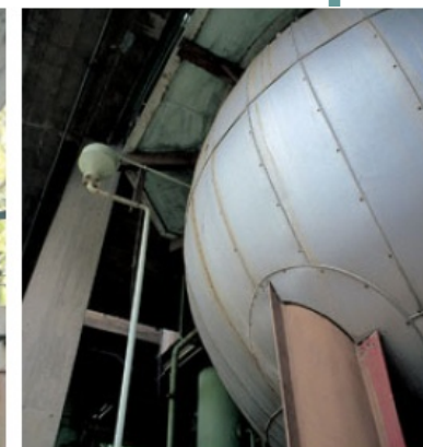
Boiler for ground cassava, where enzymes are added to degrade starch, in the preparation stage.
