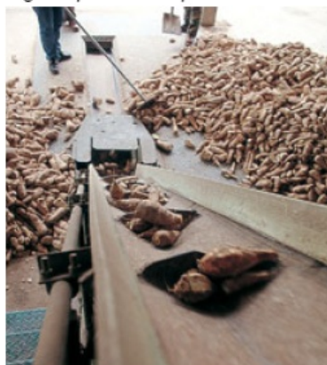
Fresh cassava with roots removed before entering the peeling equipment, a step in the preparation of raw material.
