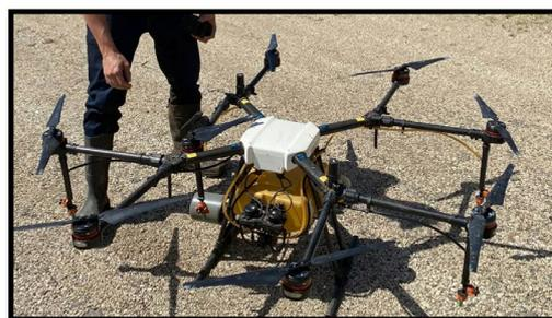
Figure 2. Unmanned aerial vehicle (UAV) used during spraying.
